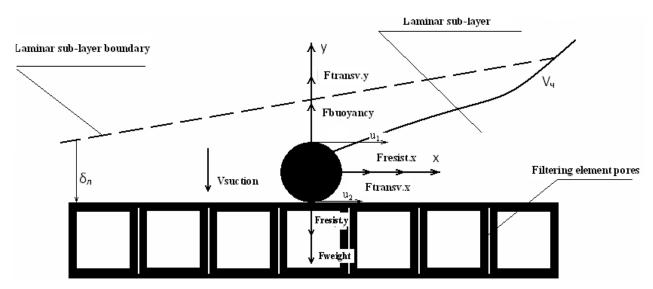
Figure 5: The forces influencing an impurity particle near the filtering surface
