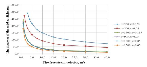
Figure 9: The calculation of a boundary size of the particles that are thrown back from the laminar sub-layer as a factor of the oncoming flow velocity at different densities of particles
