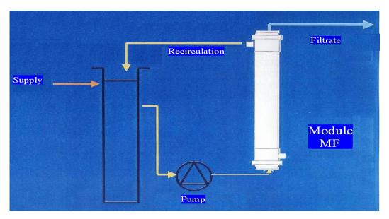
Figure 2: Main components of the equipment for classic cross-flow filtration
