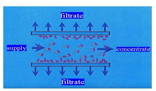
Figure 1: A basic diagram of cross-flow filtration
