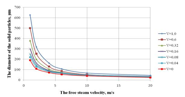
Figure 10: The calculation of a boundary size of the particles that are thrown back from the laminar sub-layer as a factor of the oncoming flow velocity at different filtration rates
