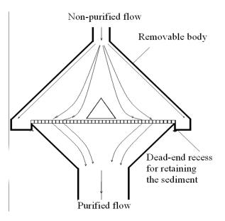
Figure 3: A cross-flow filter with a peripheral recess for retaining suspended impurities
