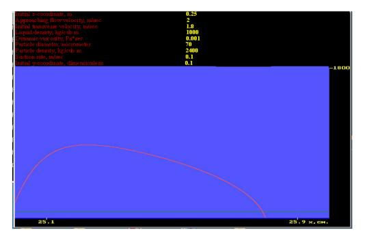
Figure 7: An example of motion of a large particle after it has torn off an obstacle provided that the suction is available
