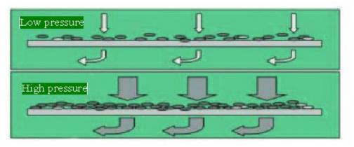
Figure 12: The effect of trans-membrane differential pressure
