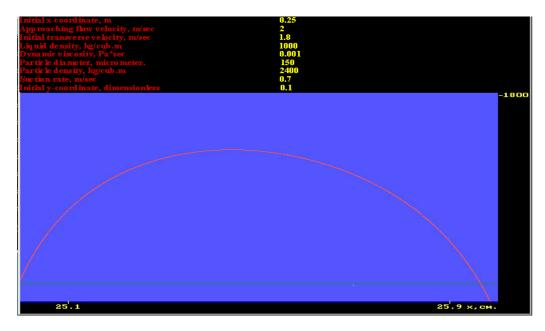
Figure 8: An example of motion of large particles (150 µm) at a considerable filtration rate (0.7 m/sec)
